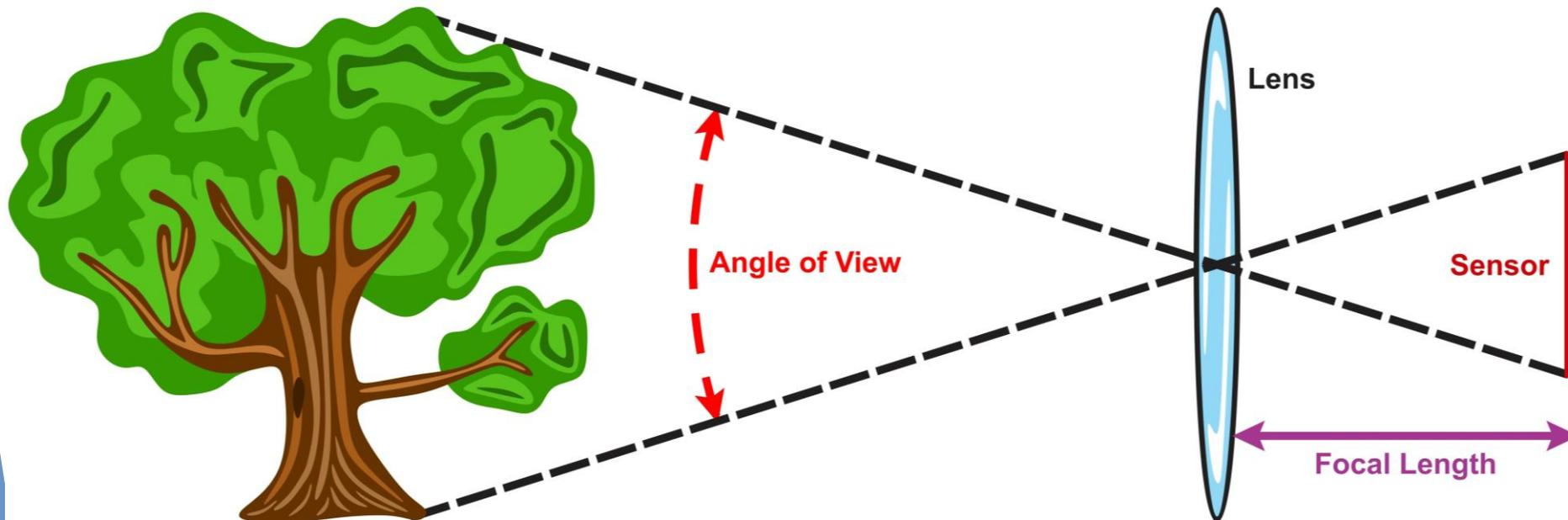
The greater the focal length, the closer the image and the less the angle of view
